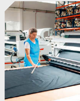
FABRIC SPREADING IN CUTTING DEPT.
